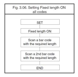
It is possible to configure a fixed length or a minimum and a maximum length for selected symbologies by reading the respective option followed by a barcode label with the required length. The different functions may be combined and will be used as follows:
